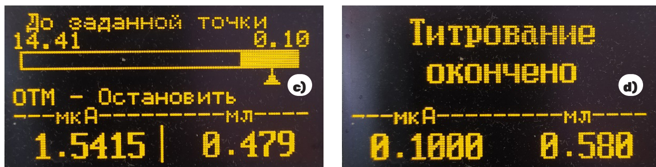
Figure 2. Data obtained at assay of a solution to be analyzed of Ferimax syrup by automatic amperometric method with two Pt indicator electrodes polarized up to 0.1 \mu\text{A} current intensity with \text{Na}_2\text{S}_2\text{O}_3 standardized solution without the addition of acetate buffer: a) at the beginning of titration; b) in the zone farthest from the equivalence point; c) in the zone near the equivalence point; d) the titrant volume at the equivalence point. ( V_0=50.0 \text{ ml} ; V_1=2.50 \text{ ml} ; m=0.8681 \text{ g} ; \rho=1.2404 \text{ g/ml} ; F=1.073 )
